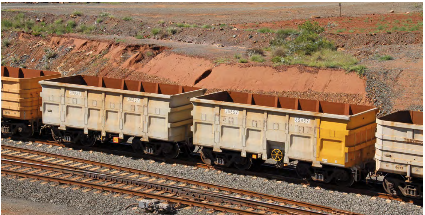
Below: A pair of empty cars 30857/35857, are seen in Cape Lambert yard 16 June 2015. The shape of the internal framing can be seen clearly, and contrasted with the narrower frames of the adjacent Bradken wagon to the right.
